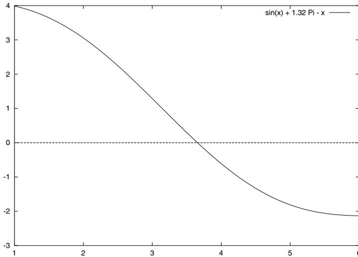
Figure 4. Example 7.2.1: Transformed Fixed-Point relation for the root finding of a one-dimensional problem.  $\alpha_0$  is the intersection point of the two graphs.
