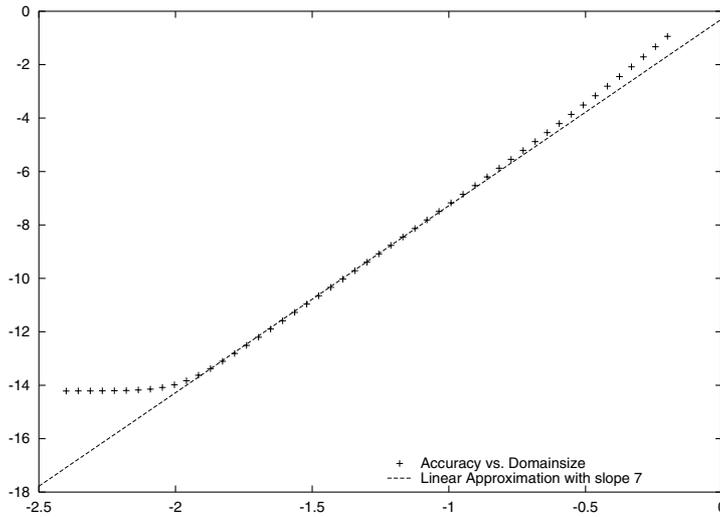
Figure 6. Example 7.2.3: Double-logarithmic plot of the accuracy of the first Newton step as a function of initial domain size; results for 6-th order Taylor models.
