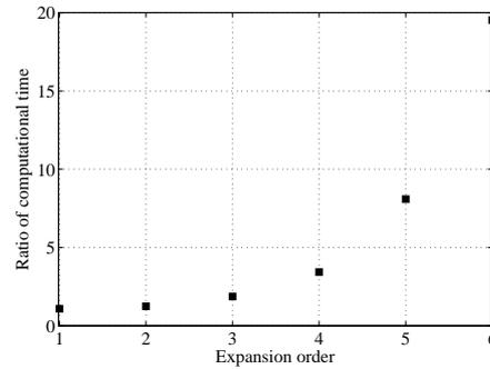
Figure 5. DA integration computational time compared to single pointwise integration.
