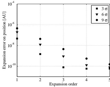
Figure 3. Accuracy of the Taylor expansion of the flow corresponding to different expansion orders and initial uncertainty sets: position error.
