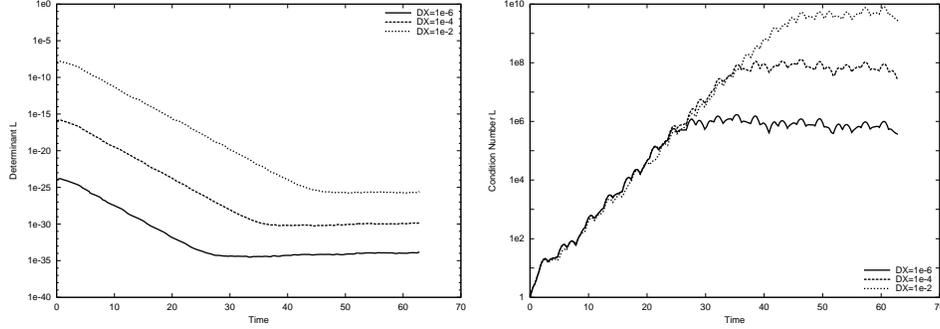
Figure 14: Simulation of the Muon Cooling Ring for initial condition boxes  $(0, 1, 1, 0) + [-d, d]^4$  located at the upper top for  $d = 10^{-2}, 10^{-4}, 10^{-6}$ . Shown are the determinants of the linear part (left) indicating progress in cooling, and the condition numbers of the linear part (right).
